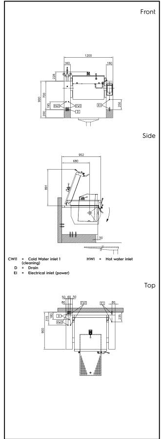
Electric Supply voltage: 400 V/3N ph/50/60 Hz Total Watts: 15.5 kW Installation: FS on concrete base;FS on feet;On base;Standing
